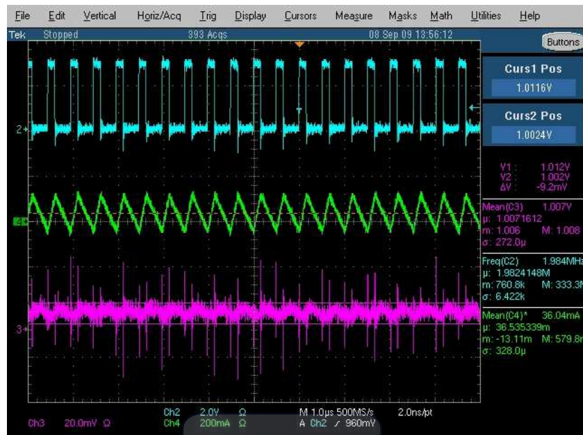
Figure 18. L=GTSD32P-2R2M, C=Ceramic 4.7 \mu F 0805 X5R TDK (Ripple 9.2mV)
