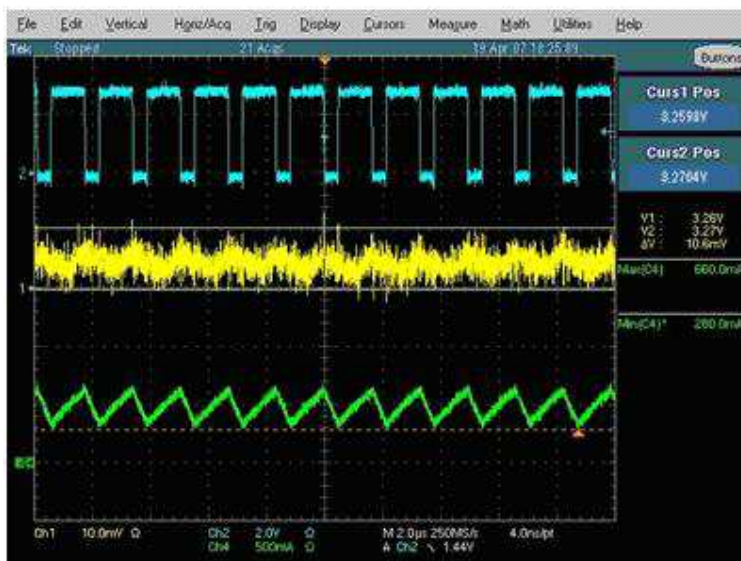
Figure 13. Ceramic 10 \mu F 0603 (X5R) (Good)
